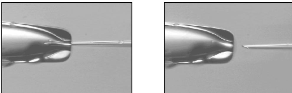
**Fig: Correctly mounted injected and holding micro pipette. The contact of the pipettes should be avoided as it may damage the injecting pipette tip.**
