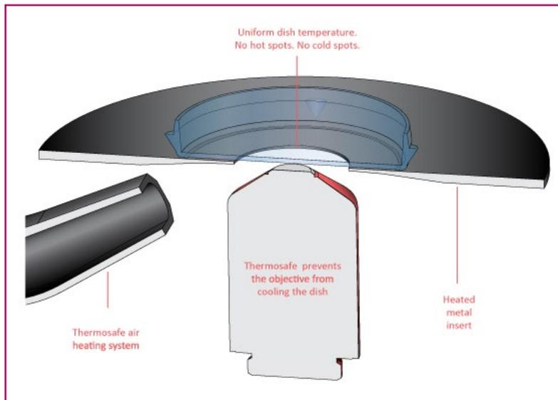
Fig 4.1: Thermosafe heating system
