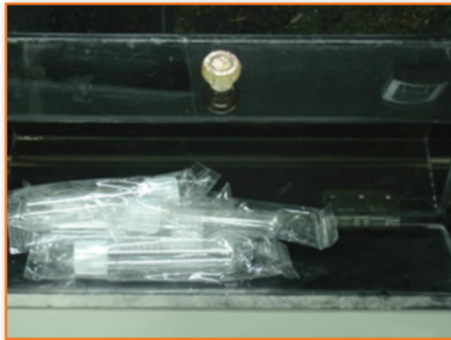
Fig: 6 Test tube warmer. For preheating of slides, petri-dishes, pipettes, etc. at desired temperatures. The dimensions of anodized aluminum heating plate are 300 mm (L) x 100 mm (W) x 40 mm (H). Bigger size plate also can be supplied with separate digital temperature controller. The temperature range is from ambient to 110^{\circ}\text{C} . The tubes are kept here just before the OPU procedure. Roughly we require 1 tube for 2-3 follicles. Only the calculated number of tubes should be opened
