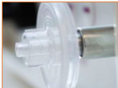
Fig: 7 Filter directly on the pump for connection with ORIGIO needle sets
