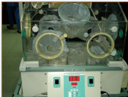
Fig: 7 A baby incubator to warm up the disposable's for the embryology laboratory. This ensures that the tubes and plates are at 37^{\circ}\text{C} before the ovum pickup procedure
