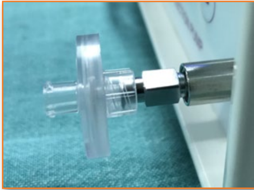
Fig: 8 Female/female adaptor and filter for connection with male tubing line sets
